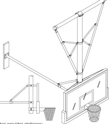
The ceiling-suspended TS-22 Basketball Backstop provides stationary installation for extreme rigidity, with a horizontal back brace attached to an adjacent wall; where folded backstops are not required. Backstops are custom designed so the lateral sway brace intersects the main mast at approximately 54" (1.37 m) above the goal and 18" (46 cm) above the backboard; to ensure maximum rigidity.
